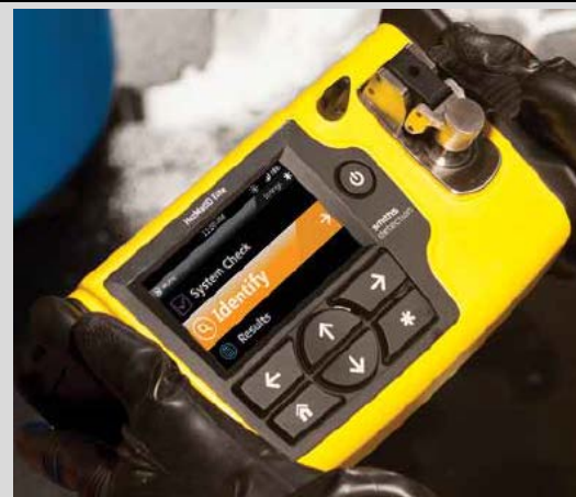
The HazMatID™ Elite is a Handheld FTIR With Integral Sample Press
